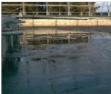
Fig.3: At four days, more clear patches are noted and the crust has dissolved into a slurry form.
