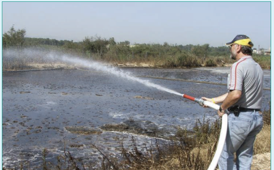
Fig.3: Treatments were mixed with water and sprayed over the surface of the lagoon to provide maximum contact with the surface oil.
